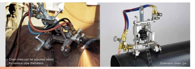
The Picle-1 is a manually operated pipe cutting machine for cutting and bevelling pipes. Equipped with a chain and worm gear drive system with low transmission ratio, leading to an absolutely frictionless feel.
