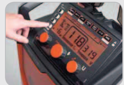
Kemppet Adaptive (A) models include special features, including power setting by plate thickness control, filler materials selection and memory channels.
