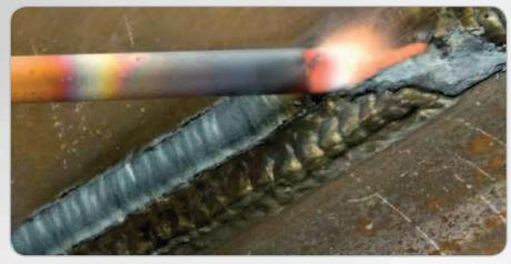
KempGouge ARC 800 makes easy work of carbon arc gouging tasks.
