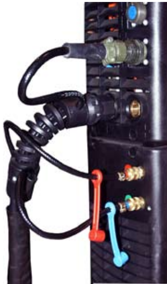
Installing water-cooled torch
